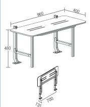
Seat size: 960 mm x 400 mm seat with 100 mm x 60 mm coved plated rear legs for fixing to floor with 10 mm front leg Acetyl plugs to suit shower cubical gradient.
